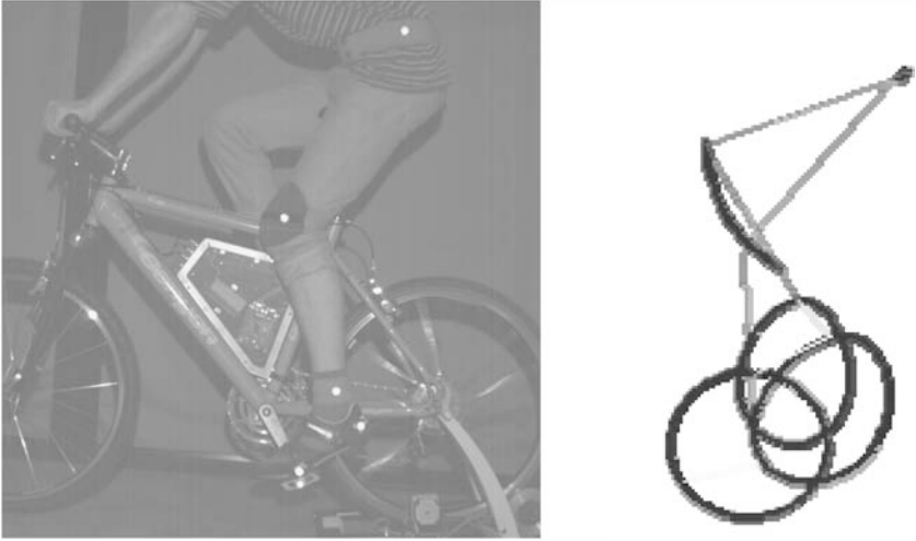
Figure 5: A single frame of a high-speed video and marker trajectories.
