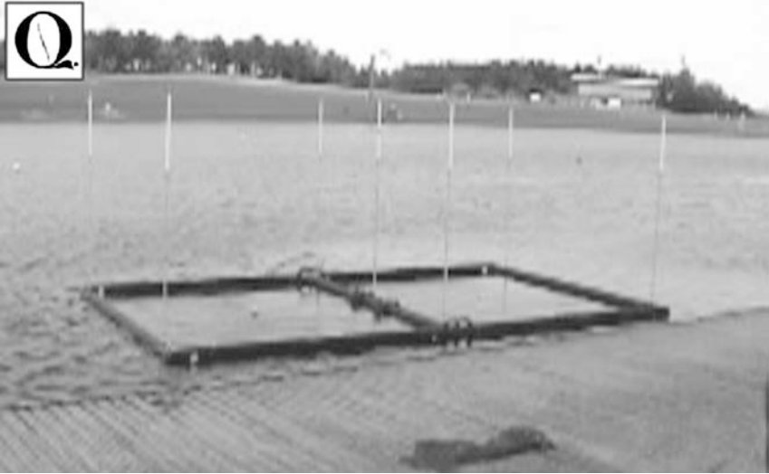
Figure 13: Illustration of a floating three-dimensional calibration frame used in kayaking research.
