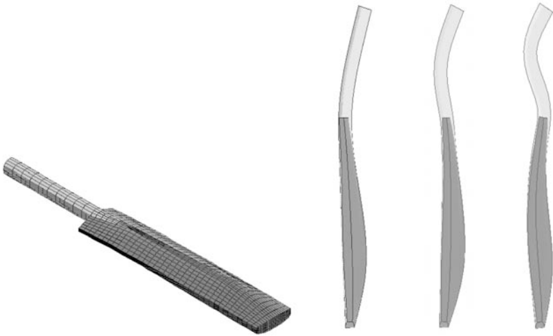
Figure 8: Computer model of the bat and its three lowest eigenmodes.
