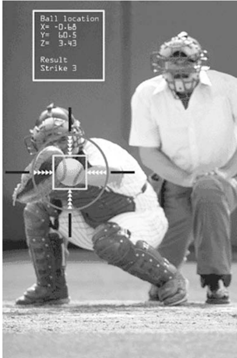
Figure 3: QuesTec video analysis system for calling balls/strikes in baseball is controversial. ( http://www.isa.org/Images/InTech/2003/July/20030761.gif )
